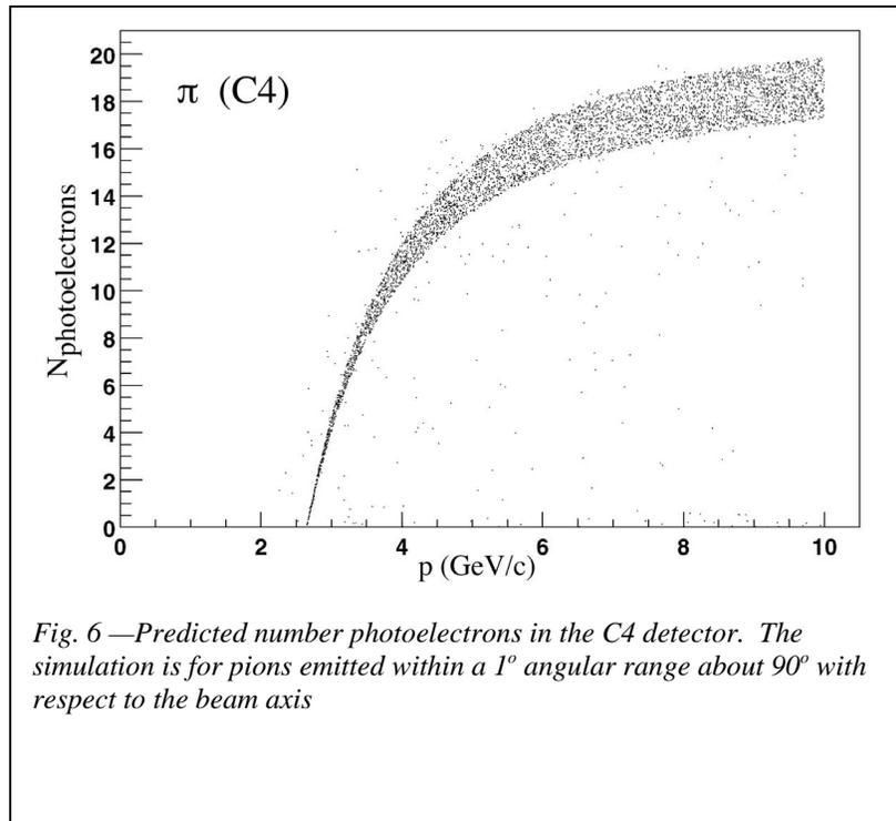
*Fig. 6—Predicted number photoelectrons in the C4 detector. The simulation is for pions emitted within a  $1^\circ$  angular range about  $90^\circ$  with respect to the beam axis*
