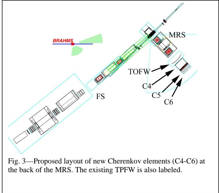
Fig. 3—Proposed layout of new Cherenkov elements (C4-C6) at the back of the MRS. The existing TPFW is also labeled.
