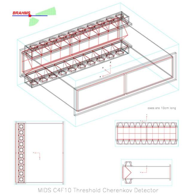
Fig. 5—Initial design study for C4 threshold Cherenkov detector.
