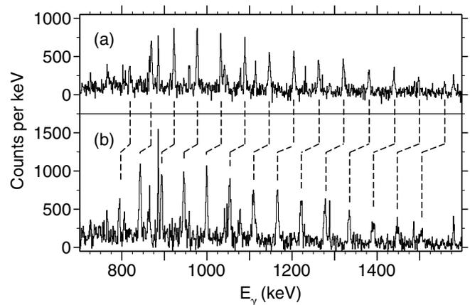
FIG. 2. Partial spectra of  $\gamma$  rays double gated by nonidentical pairs of transitions in  $^{146}\text{Gd}$  SD band 2 observed in (a) forward detectors at an average angle of  $\bar{\theta} = 41^\circ$ ; and, (b) backward detectors,  $\bar{\theta} = 142^\circ$ . Dashed lines connect Doppler-shifted  $\gamma$ -ray lines from the same SD transition.
