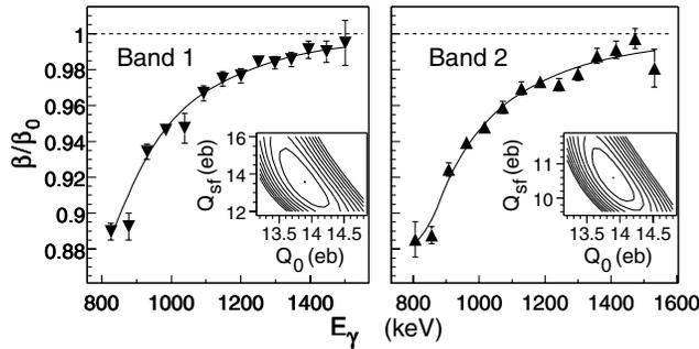
FIG. 3. Fractional Doppler shifts of  $^{146}\text{Gd}$  SD band transitions. Curves indicate the best fit to the data. Insets show absolute  $\chi^2$  surfaces as functions of  $Q_0$  and  $Q_{sf}$ . Dots in the centers indicate  $\chi^2$  minima; surrounding contours are spaced in intervals of one unit.
